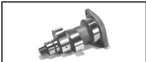
Hardfaced cam, on customer cores.
