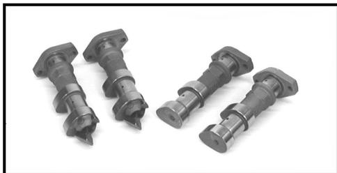
Set of 4 cams hardfaced on stock customer cores.
