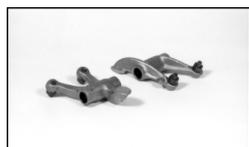
Hardfaced rocker arms are strongly recommended with all cams for these models. Stock rocker chrome has a history of failure.
