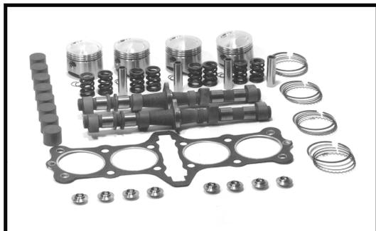
New billet cams, no exchange cores needed.
