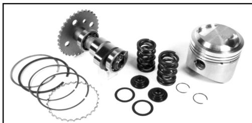
Hardfaced cam, on customer core.
