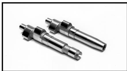
Hardfaced cams on new billet cores.
