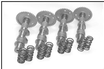
Cams (4 per set) hardfaced on customer cores.
