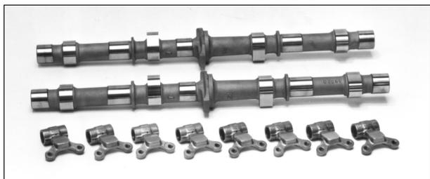
Hardfaced cams, per pair, on customer cores.
