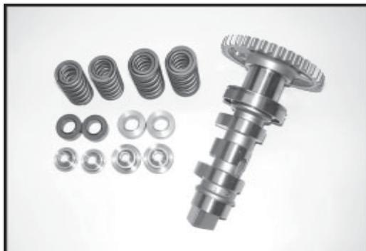
New billet cam/ no core needed. Cam will be supplied with press on flangs and adjustable cam sprocket.
