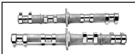
Hardfaced cams per pair, on customer cores.
