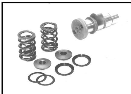
Hardfaced cam, ON CUSTOMER CORE. XR-80/100 #129-99 core charge (if no customer core).
